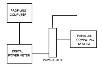
Figure 1. Experimental Set-Up for Benchmark Tests.
